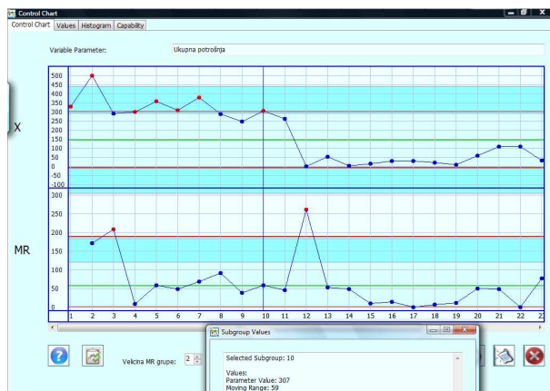
Figure 8 Individual control chart of one customer's electricity consumption in the summer period
